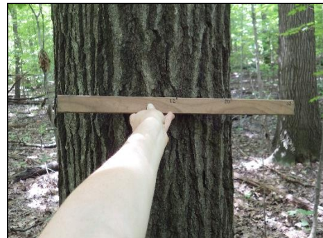
Figure 2: Using a Biltmore stick. Holding stick horizontal and ~2’ from body at ~4.5’ above the ground close one eye and visually line up the end of the stick with the left side of the trunk. This tree pictured just makes the cutoff for mature tree size.
