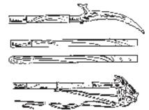
thick. A saw blade is mounted in combination with the pole pruner or may be mounted on a pole by itself. The saw is designed to cut on the pull stroke and is used to remove branches up to 4" in diameter.
